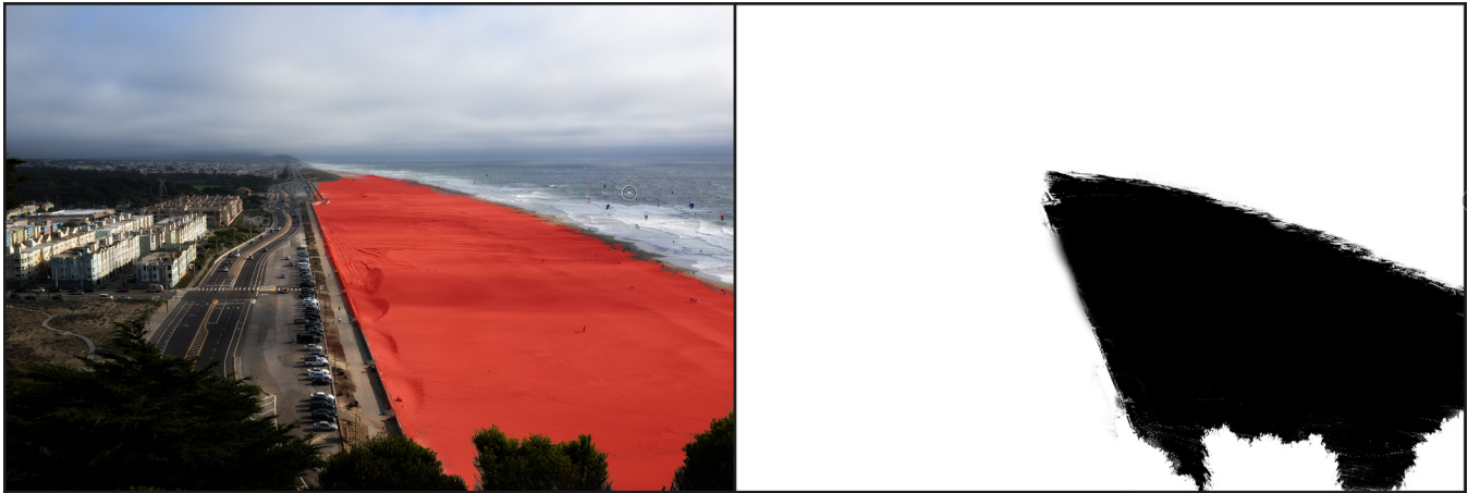
The two options for viewing a mask are with a red overlay (left), which shows the masked areas in red, and a grayscale mask (right), which shows only the mask, in a range of tones from white (not masked) to black (completely masked). Tones in gray represent varying percentages of the mask's opacity.
