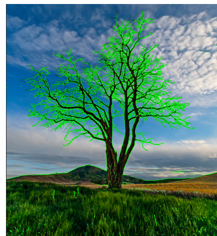
The Focus Mask option displays areas of sharpness with a bright green overlay.
