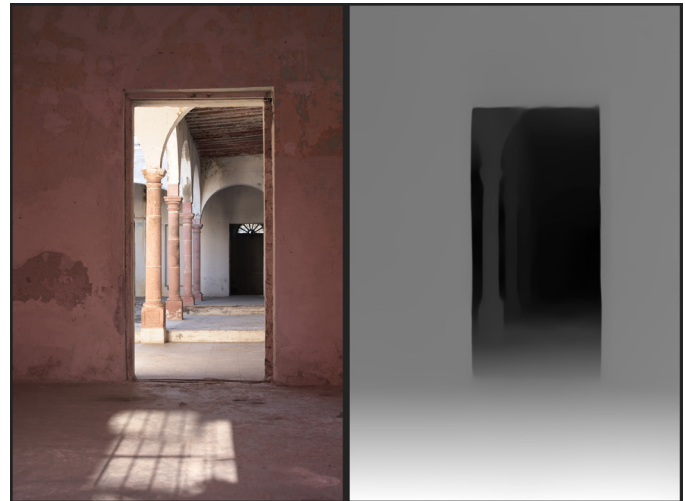
The depth mask for the photo above is shown on the right. Lighter tones are the areas closer to the camera, while darker ones are further away.
