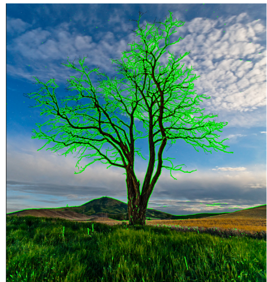
The Focus Mask option displays areas of sharpness with a bright green overlay.
